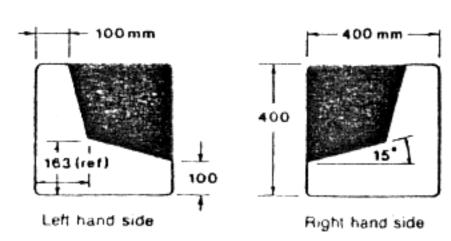
The surface of the plates must be retroreflective material which meets Australian Standard AS 1906 Class 2. (This is similar to the material used on number plates and some road signs.) Each plate must be marked with the maker's name, and the standard of reflective material. When buying a pair of plates, make sure that this information is provided on each of them.
